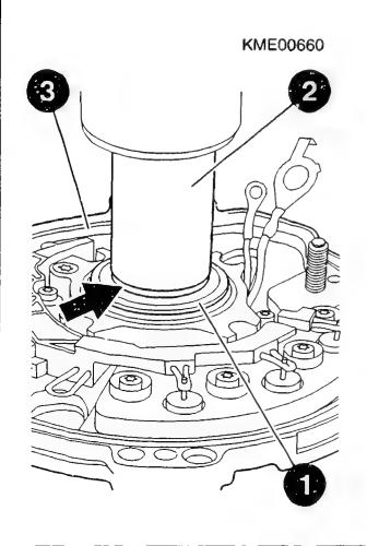
Assembling drive-end shield Use plastic spatula to apply thin coat of thermal conduction paste to contact surface (1) at housing (2). ATTENTION: Thermal conduction paste must form a continuous layer. If position is corrected, make sure contact surface at housing is completely coated with thermal conduction paste.
